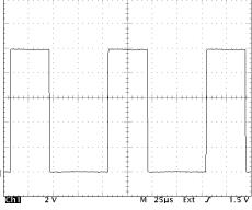
Typical Output Waveform, 10KHz, 10,000V, 120pF Load
